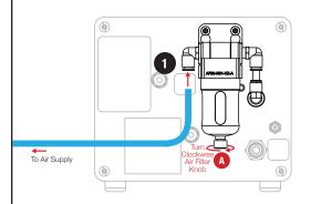
Power off engraving system and air supply. Insert hose from air supply to filter fitting marked "Air Input" (see 1) until the hose stops and is secure.
