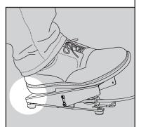
During use, foot should be completely on the foot pedal.
